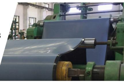
Traditionally available in smaller moulded sheets, J-Flex can now offer calendered roll products, typically 1200/1400mm wide x 10 metre long rolls (dependent upon thickness).
